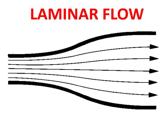
Laminar or Streamline Flow, is a well-ordered flow and is characterized by the smooth sliding of adjacent fluid layers (or lamina) over one another, with mixing between layers occurring only on a molecular level.
