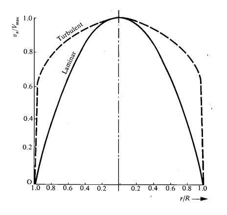
For laminar flow the velocity profile is parabolic; in turbulent flow, the curve is somewhat flattened in the middle. Notice that for both cases the velocity is the fluid-wall at zero interface, this is known as the no-slip boundary condition.
