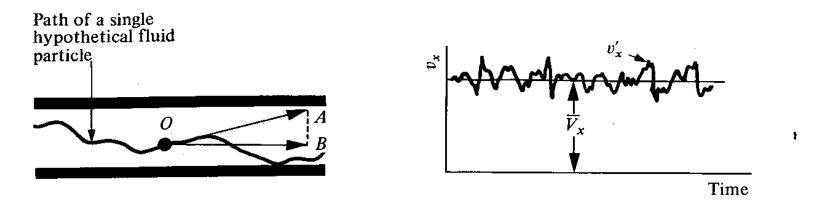
**Turbulent Flow,** is an erratic (irregular) flow and is characterized by the transfer of small packets of fluid particles between layers. Thus it is accompanied by fluctuations in velocity.
