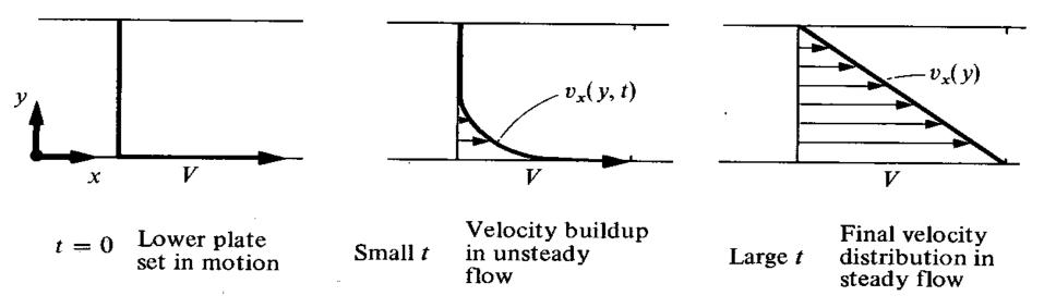
At steady state, for plates of **area A**, and laminar flow, the force is expressed by
